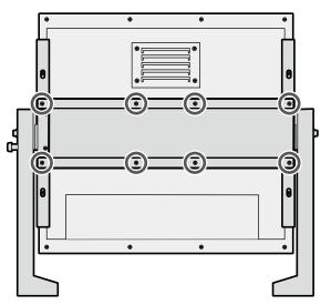
Screw: M4 x 14 Screw tightening torque: 1.0 N·m - 1.4 N·m Tool required: Phillips screwdriver (#2)
