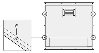
2. Fasten one of the stands by screwing the included screws into the two screw holes where the spacers have been inserted.
