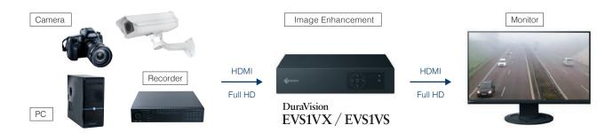
DuraVision EVS1VX and EVS1VS image optimization systems connect to a camera, recorder, or other image output device via HDMI and process incoming video content to make it easier to see. They use EIZO's unique visibility enhancement technology to analyze and process images in real time without altering the source data.
